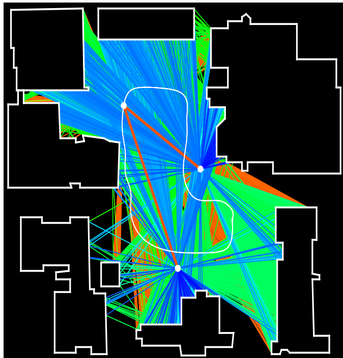
Fig. 1. An example scene as represented by the developed simulation software. This figure depicts a single simulation frame, with the buildings, transmitters, receivers, and transmitter motion path in white, and the signal rays colored by amplitude.
